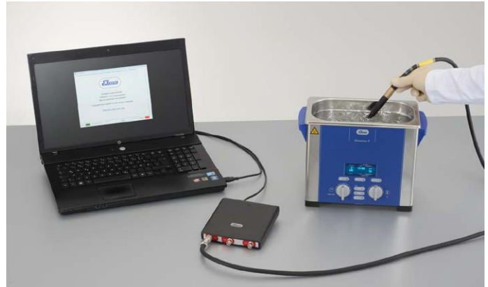
Elmasonic P 30 H during the cavimeter test
