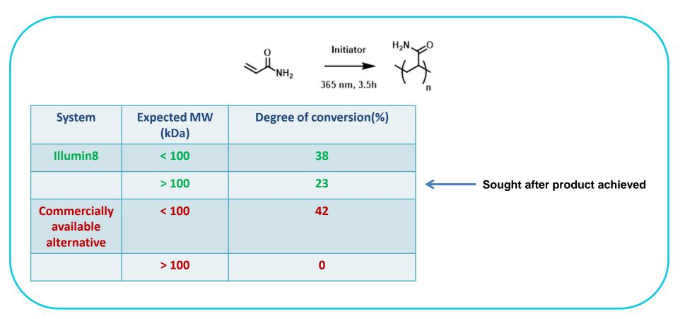
With Illumin8 high MW polymer can be obtained (conversion based on NMR data, need confirmation by GPC). Using the UVP chamber no conversion was ever obtained for MW > 100 kDa.
