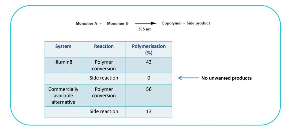
With Illumin8 the temperature of the solution after irradiation was 28 °C while with the UV chamber and no cooling system was  $\approx$  40 °C. The higher temperature can explain the degradation of the allyl double bond which is unwanted and yields side products.
