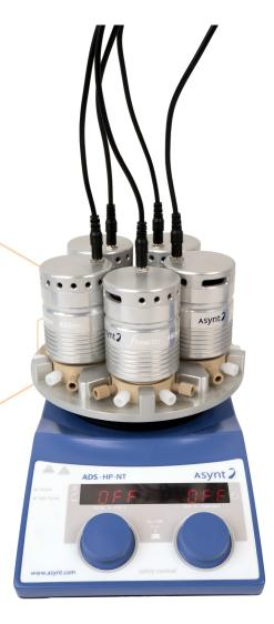
Heating and agitation is provided by any magnetic hotplate stirrer.
